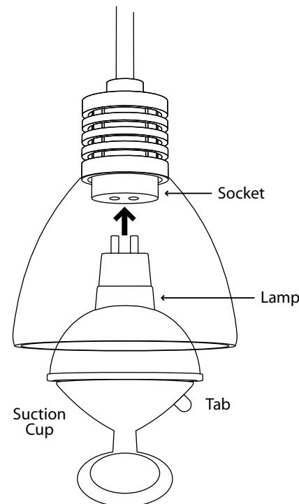
**4** Remove the suction cup by pulling on the tab.
