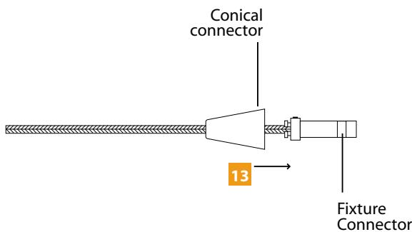
**13** Slide the conical connector over the fixture connector. To install the fixture, refer to the instructions provided with the system.
